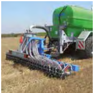
Slurry injector Innovative spreading technology
