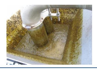
4NHTB Manure Pump High Head Solids Handling Pump Max. 450 m³/hour, Max. 140 mwc
