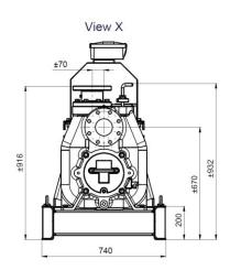
6STX - 37 kW motor - frame total net weight 975 kg
