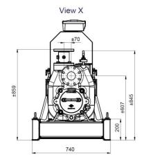
4STX - 22 kW motor - frame total net weight 750 kg
