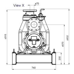
6STX - 30 kW motor - frame total net weight 850 kg
